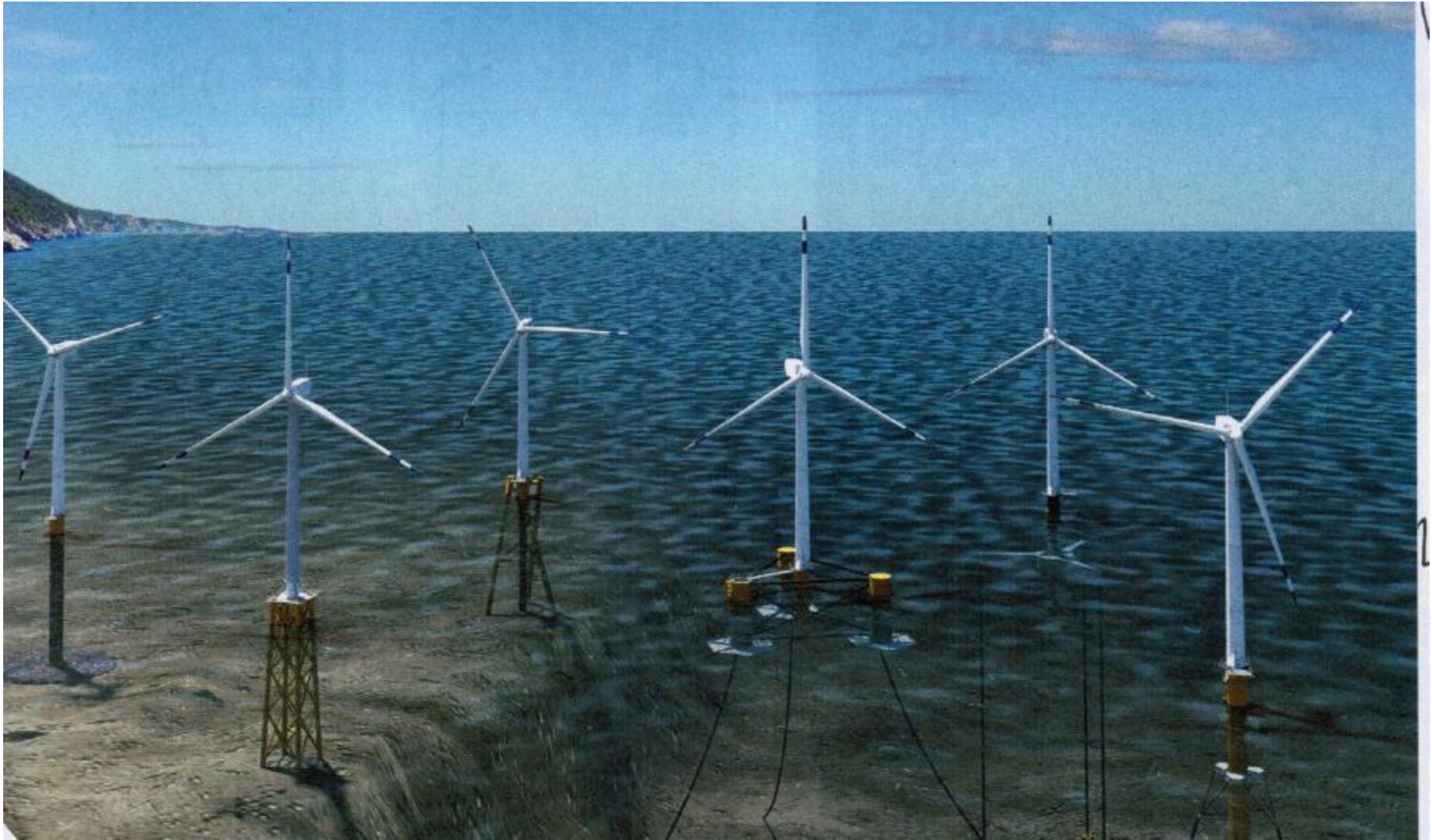
Left turbines on continental shelf; right turbines cabled to ocean floor.
