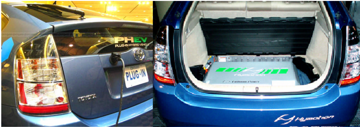
Figure 3-30. The Hymotion plug-in module for the 2004-6 Toyota Prius.
