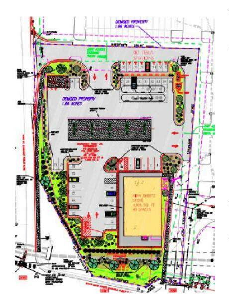
The 8 Supercharger stalls are in the upper right corner; they are outside the store and gasoline pumps area, which should help prevent <a href="ICEing">ICEing</a>.
