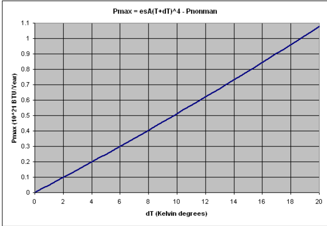
Figure 2. Limit on nonrenewable energy use by humans as a function of the change in the average surface temperature ( dT ) from year 2000 of the Earth due to that additional heat energy source.
