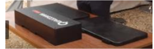
2 charge pads and charge controller in car
